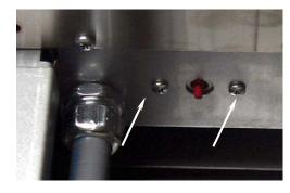
Remove screws (arrows) securing high-limit to fryer.
